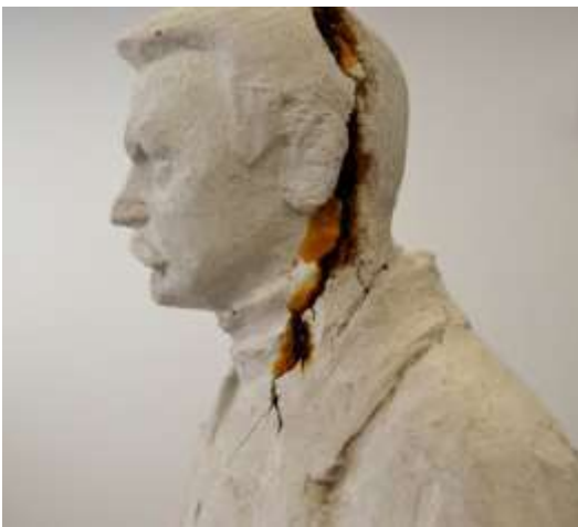
Photo 4. Small figure Edelfelt with broken parts due to oxidation of iron structure.
